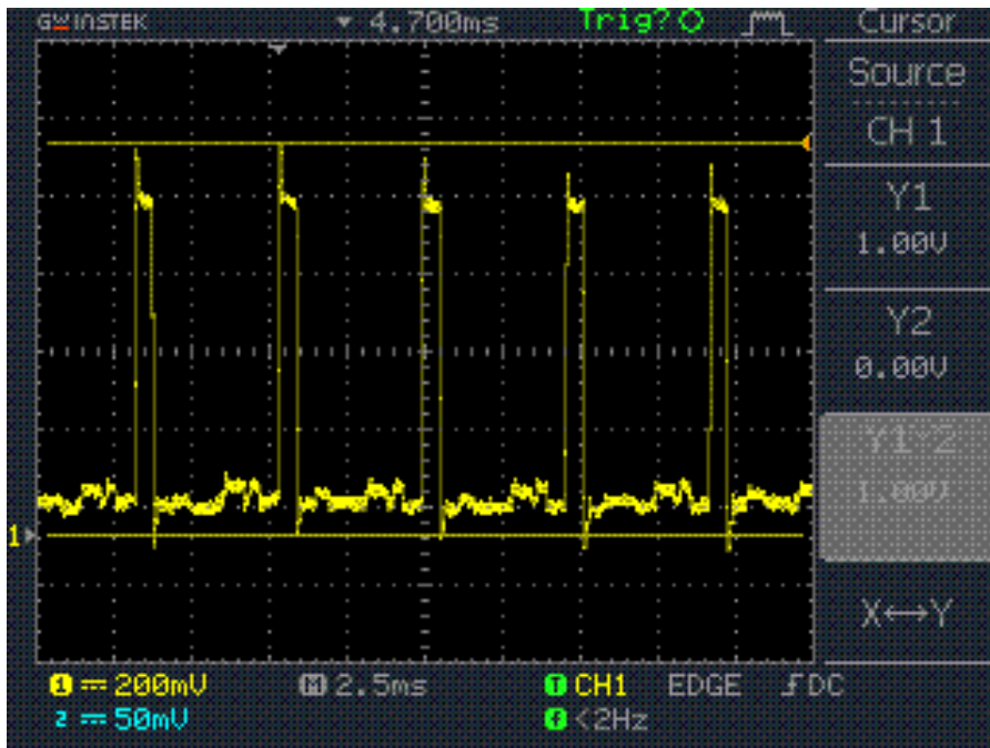
Figure 1: The GSM burst peak current of GGB-1916 is 1A in this case. The pulse is 577uS.
